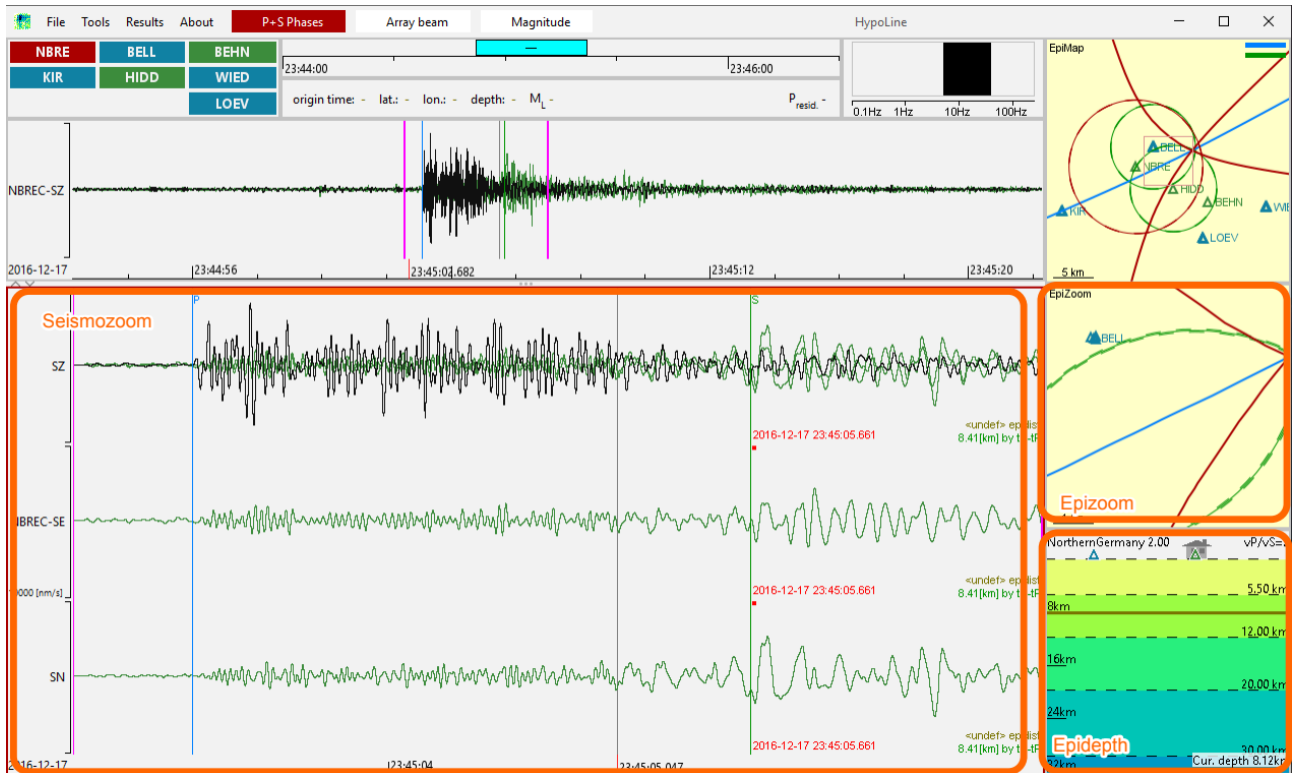
Figure 2: “P+S Phases” mode with station NBRE selected. The annotated elements are unique to this mode.
